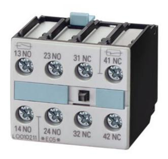
ELECTRONICS COMPAT. AUX. SWITCH DIN EN 50005, 1NO+1NC (ENCLOSED) A.1NO+1NC (NON-ENCLOSED) SIZE S0...S3
