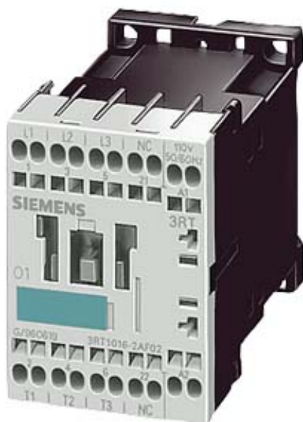
CONTACTOR, AC-3 3 KW/400 V, 1 NO, AC 24 V, 50/60 HZ, 3-POLE, SIZE S00, CAGE CLAMP CONNECTION
